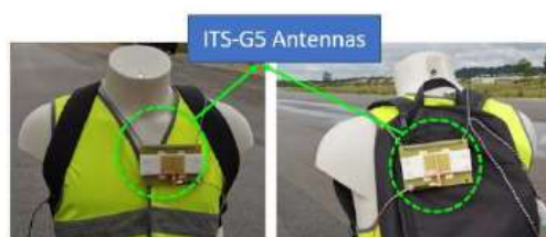
Antenna for roadworker safety application (©Uni Eiffel)
